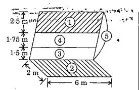
With reference to the above figure, the shape factor between 1 and 2 is
