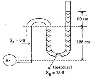
(Where  $S_A$  and  $S_B$  are the specific gravities of the two fluids)
